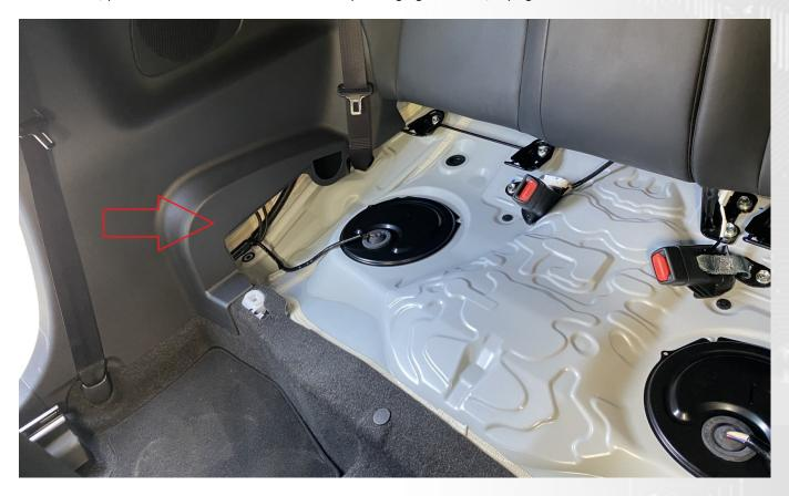
Unplug and remove OEM Controller, bolt the Syvecs Yaris AWD Unit in its place
