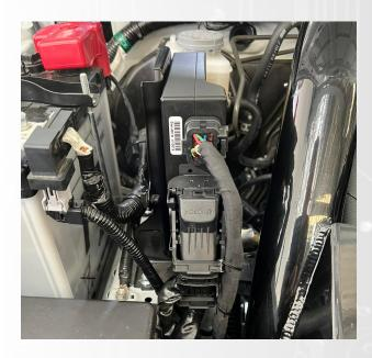
7 Remove the OEM Lambda Sensor and replace with the NTK Lambda supplied. Important! make sure the sensor is mounted vertically.Connect the Lambda Loom from the 26Way connector into the NTK lambda.
