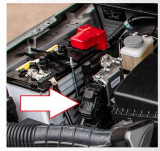
${\tt 3}$  Unbolt the Factory Engine ECU and remove from the engine bay.
