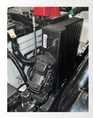
$6\,$  Plug in the 26Way connector into the front of the Jimny Plug in ECU, this will allow for connection to the ECU via ethernet.
