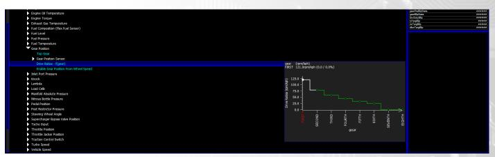
Flat Shifting - When the Clutch is pressed on it will send a GearCut Request into the ECU for Flat Shifting. This is Setup in Gearcut - Open Loop
