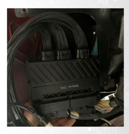
6.) Mount the Ecu with bracket provided and secure using the M6 Bolts. The washers should be fitted behind the bracket to space it out towards the wheel 4mm, this allows the adaptor to fit correctly behind the Syvecs ecu.
