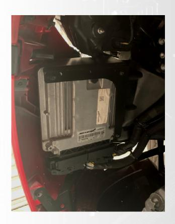
5.) Connect the Syvecs 720 adaptor and wiring loom between the ECU and Adaptor box. (Pay attention to the engravings on the connectors and boards to show which way round it is connected)
