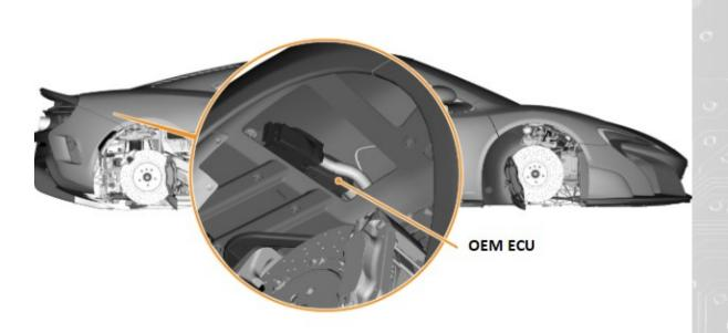
3. ) Unplug the Ecu Connectors and remove the OEM Ecu hanger complete with the factory unit
