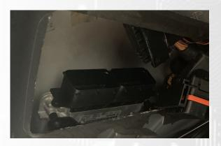
4.) Mount the S7Plus ECU in the Factory Hanger using the adapter plate and then refit it back inside the wheel arch
