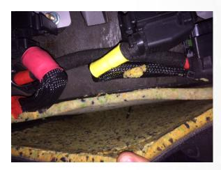
6.) After securing the ecu and associated wires head down to the passenger area footwell. Remove the carpet piece and loosen the 4 screws shown below to expose the GFA Unit
