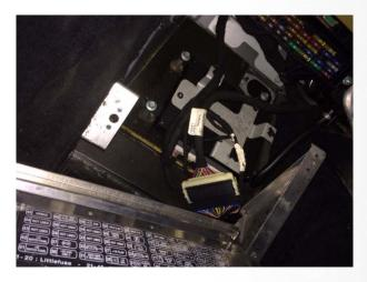
7.) Unplug the 4 connectors into the GFA and fit the Syvecs GFA Module in-between the loom and the GFA Module as shown below
