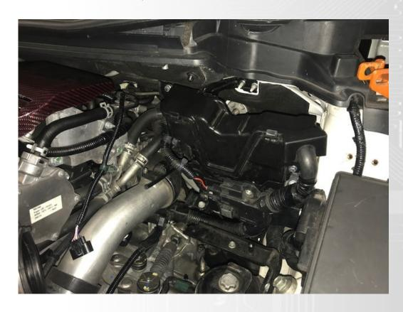
3.) Remove the OEM Engine Management Computer which is found on the right-hand side near the firewall as you're looking toward the engine bay as seen here
