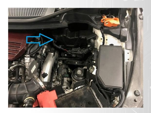
The ECU is quite easy to remove, if you are struggling to remove the ECU, make sure all the bolts have been removed and the clips holding the loom have been removed as well
