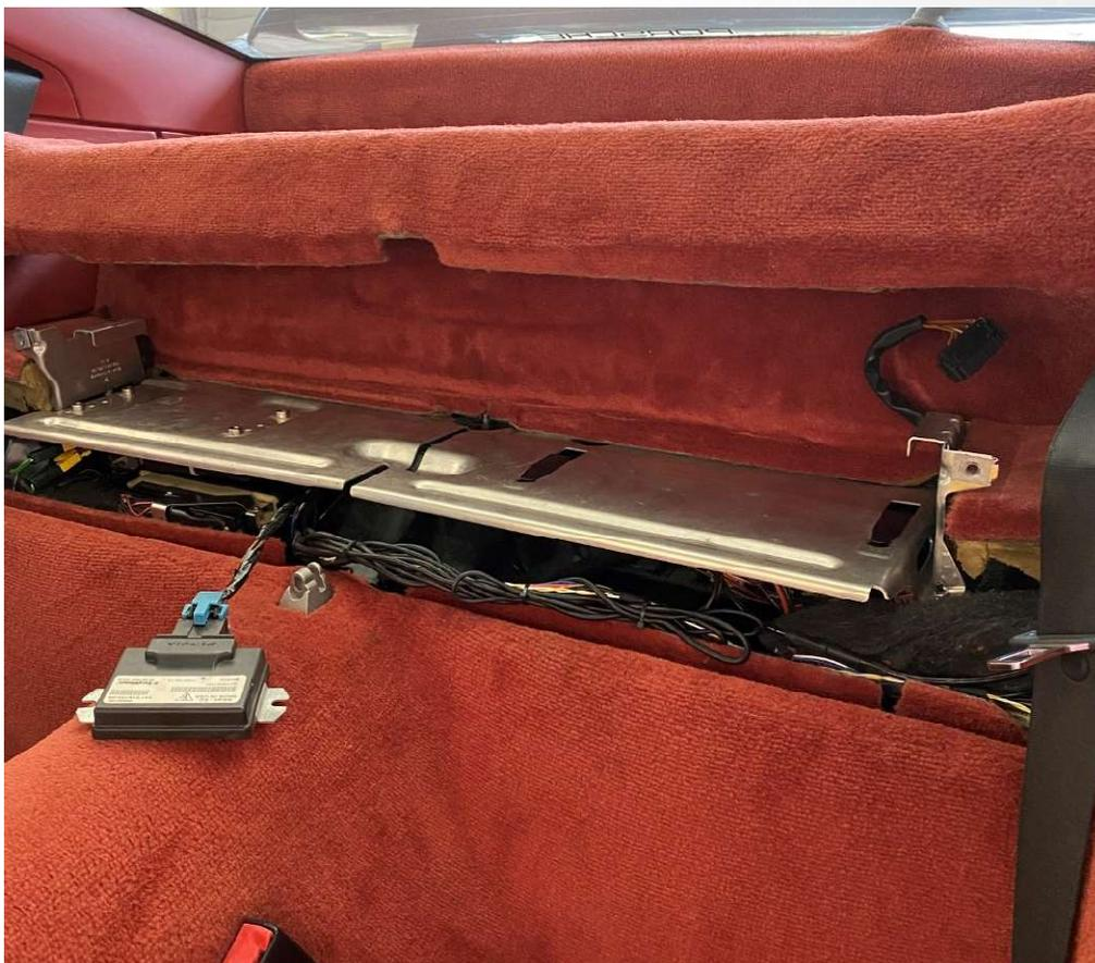
Once the carpet is lifted, remove the left ecu holder and you will find the OEM AWD Ecu on top of the OEM Engine Ecu, unplug it and remove.
