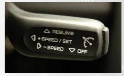
Pushing the stalk button down towards the Off Symbol and holding is used to go back down the Calibration switch positions.
