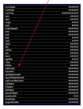
First pressing the cruise cruise button the end of the stalk will put the car into map switching mode which flashes the cruise control light on the dash. When in this mode pushing the Resume button on the steering wheel up and holding for 2 seconds will make the calibration switch go up by one value each time its pressed and held. As default there are 8 calibration switch options and the user can then assign many tasks to each calibration switch under the Calibration switches section of Scal.
