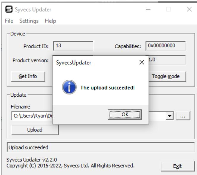
If the Upload Succeeded message doesn't appear then check that windows has not incorrectly recognized the device in device manager.
