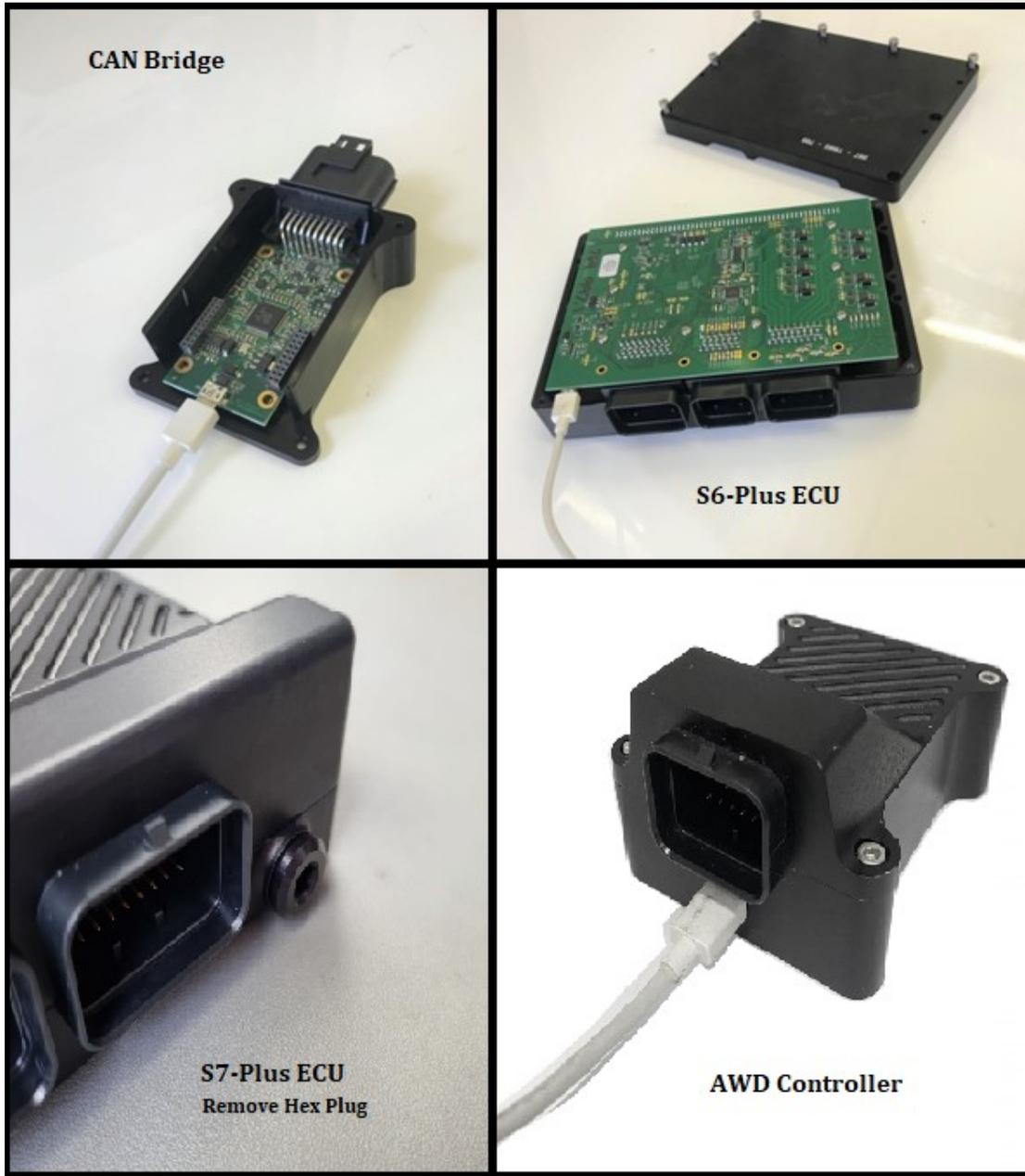
The USB cable will provide power to the devices from the computer; they do not need an external power to be connected for updating unless it's an S6-I or S6-Plus ECU which will require a 12v and ground connection. After powering up the S6-I / Plus users need to wait 10 seconds for it to enter Boot mode.
