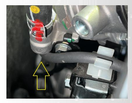
9 Forced induction applications can wire in the supplied air temp also on the charge pipe into the engine, if not turbo then the OEM air sensor in the intake air pipe can be used.
