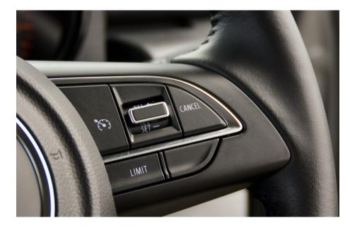
The Cruise Control buttons are used for the Cruise Strategy but also map switching. When the engine is running the Tacho will show the position on the RPM gauge when changing calibration position. Example: Cal1 = 1000rpm, Cal2 = 2000rpm
