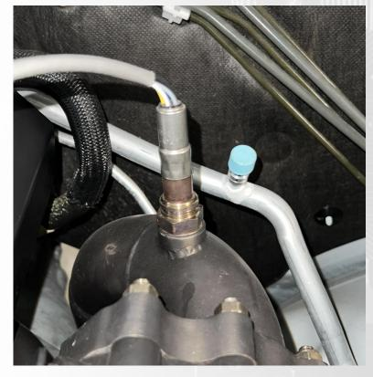
8 The 4bar Map sensor needs to connect to a vacuum source on the intake manifold
