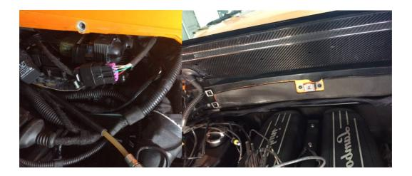
6.) Plug in the 2 Injector Looms as shown below - MUST PLUG INTO BLACK CONNECTORS - NOT BROWN
