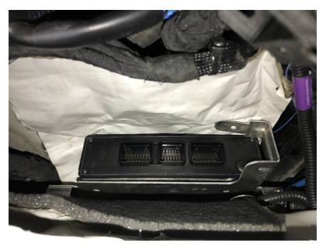
7.) Plug in the Loom and secure carefully
