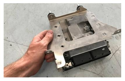
4.) Remove the 6 x Hex bolts to remove the Oem ECU from its cradle
