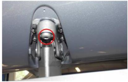
4.) Lift the top Spoiler of the legs and then slide the bottom part of the spoiler up and over the legs also
