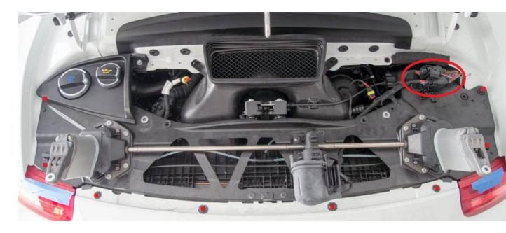
3.) Remove the Factory Ecu by removing the 2x 10mm nuts holding it in place
