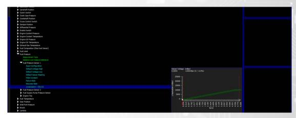
Select the Linearisation area of the Sensor setup and then again select the linearisation option in the top right hand corner of the screen. As Shown below
