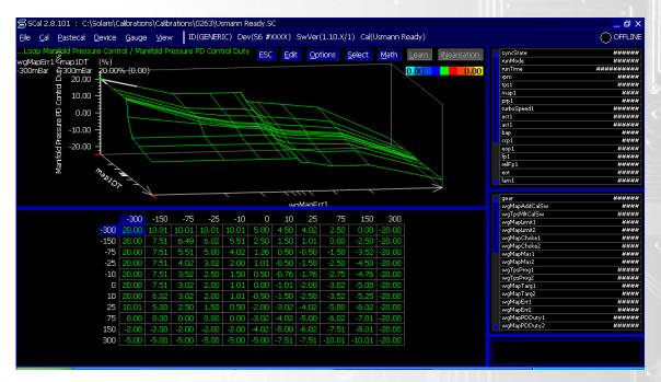
The wastegate Target and Duty can be also adjusted via the Cal Switch so be sure to populate the wastegate control Cal switch settings as you see fit. See Figure 0-10a.
