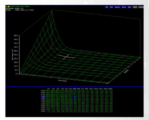
After setting the allowed slip users need to setup the torque limiting area of the strategy, fuel cuts is the easiest to understand as a 50% fuel cut results in a 50% reduction in torque in most applications but fuel cuts in a forced induction car can reduce turbine energy hugely and have a much larger effect of torque after the reduction request disappears compared to ignition retard reductions.
