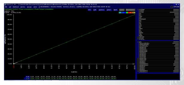
For External wastegate the Linearization should be set as below when using the Syvecs valve plumbed in as shown in *Wastegate Solenoid Fitting*.
