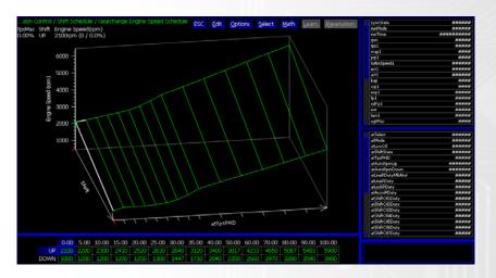
If users find that the Rpm Delta is large on some gear up exchanges that it causes the *atAutorpm down* value to be reach and request a down shift then setting a value around 500ms in the **Post-Shift Disable time** calibration found under the main gearbox control section to stop shift request until the RPM has stabilised
