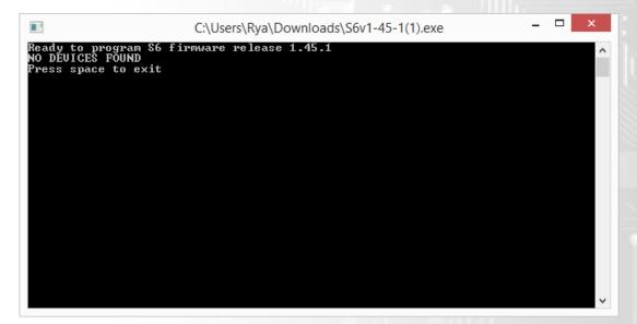
Now reconnect the Ethernet cable to the ECU and open SCfg – Click Device – Get Config Once loaded, click change software version. Select the Latest Firmware you have just ran the .exe for and then once changed click File/Save and rename so you can reload later.
