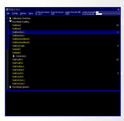
To remove the current parameter from logging, double click on the item and then leave the value empty or enter 0 in the Sampling rate command box.
