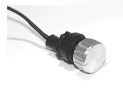
Once wired in as instructed in the Connections and wiring sections of this manual you can then see the current Calibration, Launch or Traction Switch position via the Parameters CalSelect, TcSelect or LaunchSelectSwitch found on the right hand side of the Calibration tree. See below
