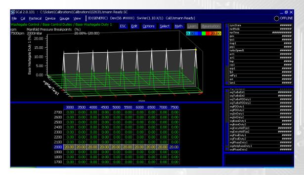
A good rule is starting at the lowest desired boost and working up and then setting everything above the maximum manifold pressure required to the same duty as that row, as shown below.
