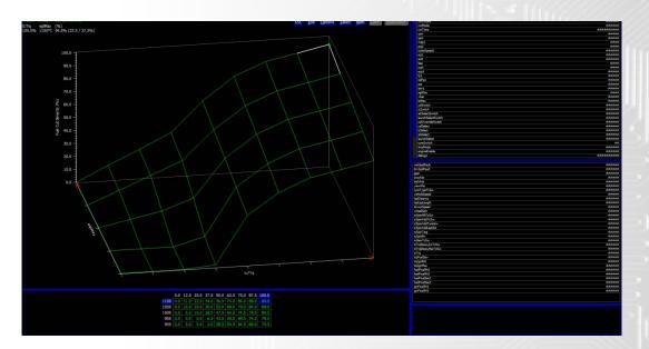
Once Torque is under control you can tweak the gain to adjust the levels of TcTrq calculated based on vehicle speed to make the system more or less sensitive. Generally its set more sensitive at high speeds where lose of traction can carry a lot more energy in the movement of the car.
