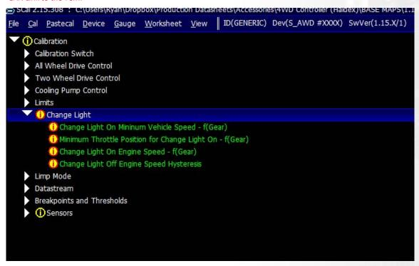
Output4 on the R8/Huracan AWD unit is the pin for the Changelight and it is found on the 12way Oem Connector -
