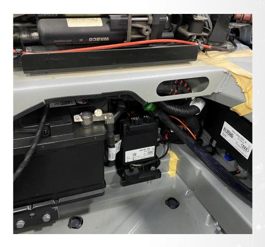
When mounting the Syvecs AWD Ecu it's best to plug in the USB Cable at the same time and route the cable into the trunk if you are planning to do live communication with the Unit. The USB port is found by removing the plug on the front of the unit as marked below.
