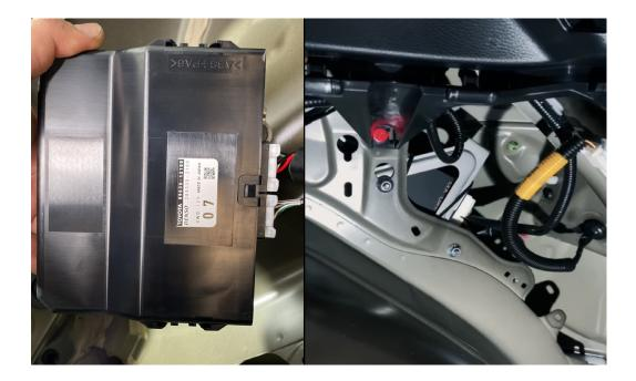
When mounting the Syvecs AWD Ecu it's best to plug in the USB Cable at the same time and route the cable into the front if you are planning to do live communication with the Unit. The USBC port is found at the back connector
