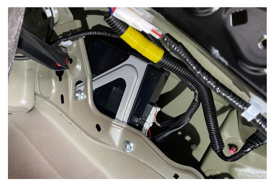
Unplug and remove OEM Controller, mount the Syvecs CorollaGR AWD Unit in its place and secure with cable ties
