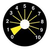
0 -1 = No Adjustment (Logic Off) 1 -2 = 0.6 Multiplier (Less Duty) 2 -3 = 0.7 Multiplier 3 -4 = 0.8 Multiplier 4 -5 = 0.9 Multiplier 5 -6 = 1.0 Multiplier (No Adjustment) 6 -7 = 1.1 Multiplier 7 -8 = 1.2 Multiplier 8 -9 = 1.3 Multiplier 9-10 = 1.4 Multiplier (More Duty)
