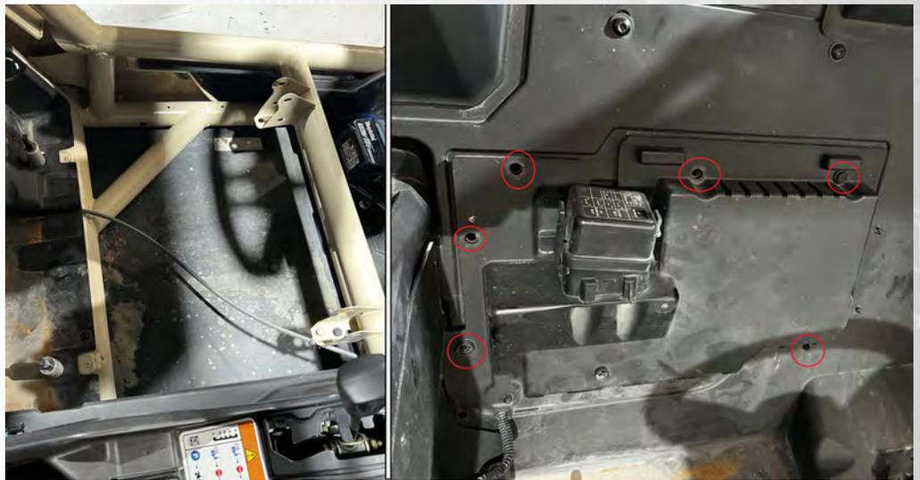
3 Remove the OEM ECU Cover and unscrew the Fuse Box from the OEM cover as this will be screwed into the new Syvecs ECU Cover.
