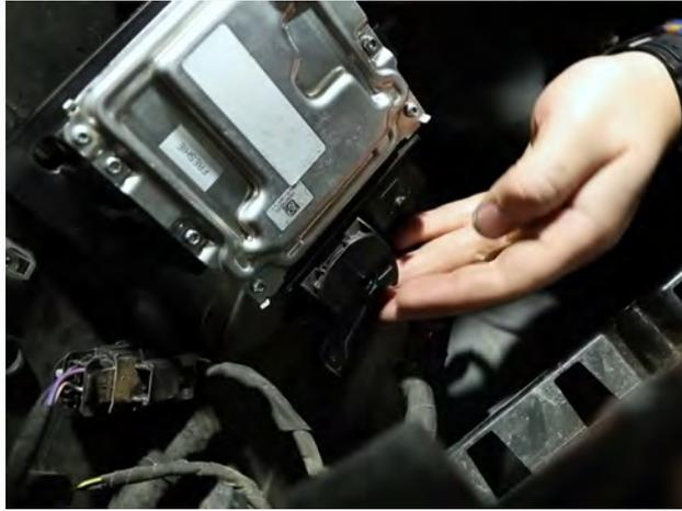
5 Bolt the Syvecs ECU in the supplied Alu cover and mount the fuse box on the new cover also. The Fuse box gets fitted 90 degrees compared to the OEM Cover.
