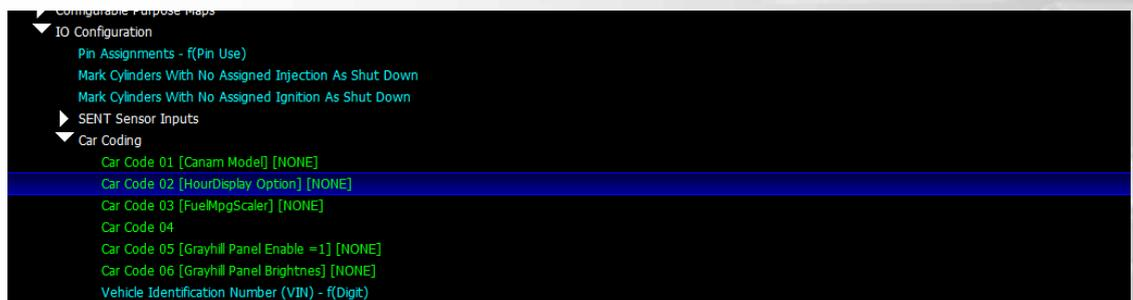
If setting up as Run Hours then the accumulated hour is stored in the ECU and not the dash. To match up the hours used to the OEM ecu you can adjust the hour offset in the below calibration.
