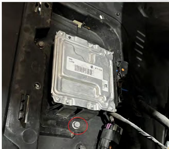
4 The Factory ECU can then be unplugged from the OEM harness and removed
