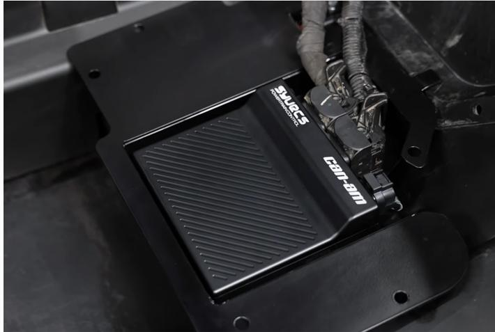
6 Plug in the 26Way connector into the back of the Syvecs Canam Ecu and then mount back the cover in the OEM Location as shown below.
