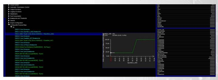
CarCode1 found in the pin assignments section of Scal is for the DPS Coding. Most models are set to 0 but we have found some models in the middle east to use Code 8. In which case put the Value 8 in this Cal if your DPS has an Error and not working
