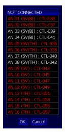
If the desired input pinout is currently allocated then it will be displayed in RED. The WHITE items show free spaces
