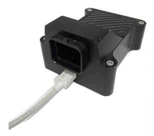
The AWD Unit will come pre loaded with a base calibration that has default values which simulate an OEM AWD unit. Use Syvecs Scal software to adjust. See last Page
