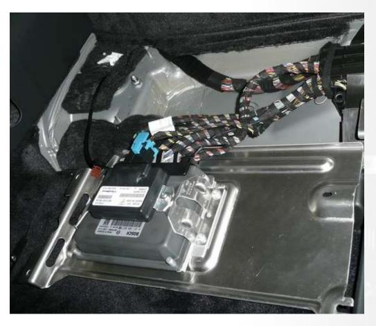
Unplug and remove OEM Controller, replace with the Syvecs 997 AWD Unit in its place by securing with double sided tape or Ties
