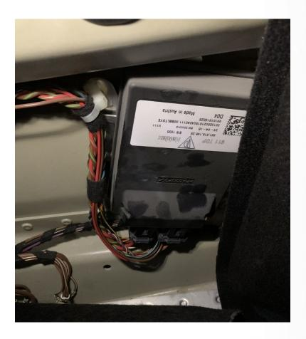
When mounting the Syvecs AWD Ecu it's best to plug in the USB Cable at the same time and route the cable into the trunk if you are planning to do live communication with the Unit. The USB port is found by removing the plug on the front of the unit as marked below.
