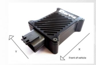
In applications where heavy vibrations are present due to solid engine mounts etc, it is advised to mount the GPS using some rubber washers to absorb some of the vibrations.
