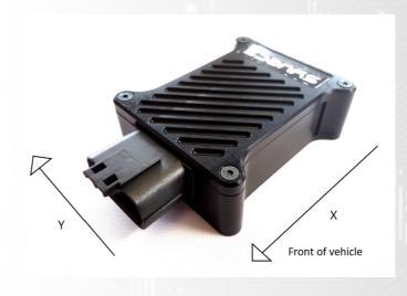
The Syvecs 50hz GPS Module is designed to provide even more control to our engine control units with accurate global positioning, acceleration forces for 6 axis and GPS Speed. Fast positioning lock with hot restarts due to internal battery storing last positioning data.
