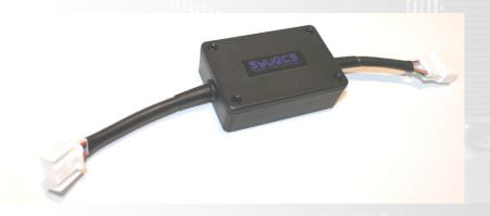
Syvecs R35GTR 4WD Controller was designed for purely motorsport use, allowing owners to get round the sudden lose of 4wd on the race track which has caused at least one big accident in motorsport. It also allows drag users to put the R35GTR into rear wheel drive mode for a short burnout to get tyres warm and clean.
