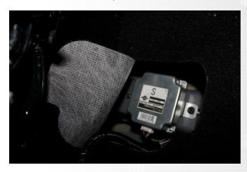
Unplug the connector going into the ecu and then plug into the female connector housing on the Syvecs 4WD Module.
