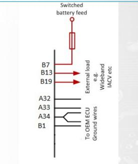
Figure 0-1 - Redundant Power Feeds and a Common grounding point.
