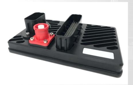
High power motorsport Power Distribution Unit (PDU). Combines a robust billet aluminium case and the very latest power driving technology with the highest efficiency in the industry. A total of 34 output channels with a max current capacity of 350A
