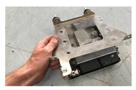
4.) Remove the 6 x Hex bolts to remove the Oem ECU from its cradle  $\,$
